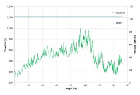
Figure 2, Pipeline profile and MAOP
