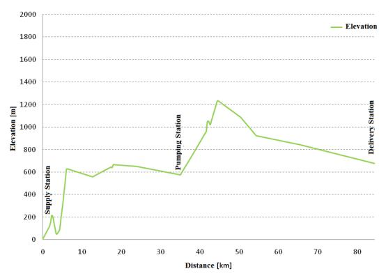
Figure 1. Elevation Profile for the VISC 30 Pipeline
