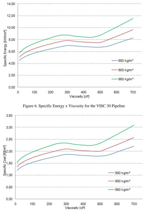
Figure 7. Specific Cost x Viscosity for the VISC 30 Pipeline
