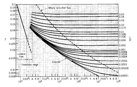
Figure 4 illustrates this phenomenon. The transition zone is approximately between 2300 and 4000 Reynolds.
