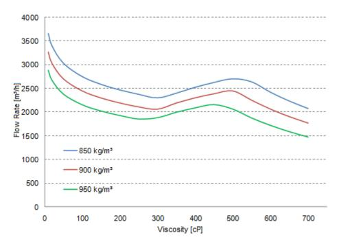
Figure 3. Flow Rate x Viscosity for the VISC 30 Pipeline
