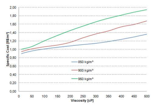
Figure 9. Specific Cost x Viscosity for the VISC 42 Pipeline
