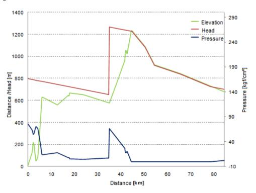
Figure 2. Typical Head, Pressure and Elevation Profile of the VISC 30 Pipeline
